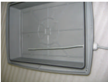
Figure 5. Insert cable through gland
