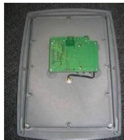
Figure 3. Attach electronics to back of lid and connect the antenna
