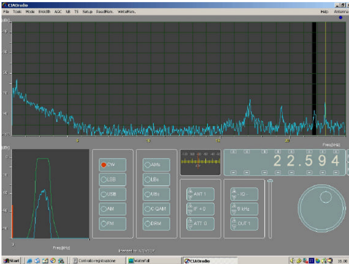
Fig 3 : Signals received in the Lab with the L101 Active loop in the 0-24 KHz band .
