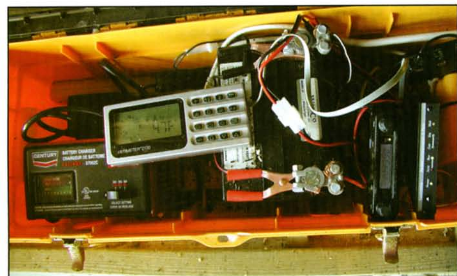
The interior of the toolbox holding the Peet weather console, 2 meter transceiver, TNC, battery and battery charger.
