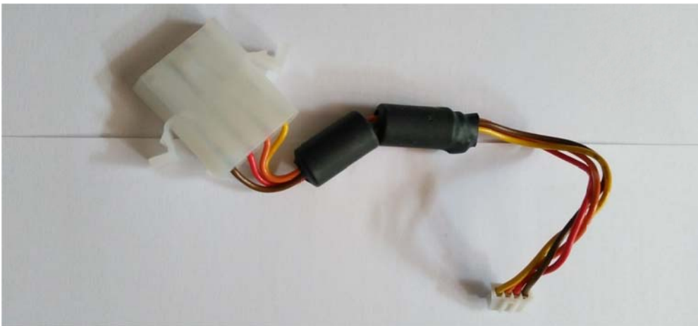
Removed Tuner Cable Assembly
