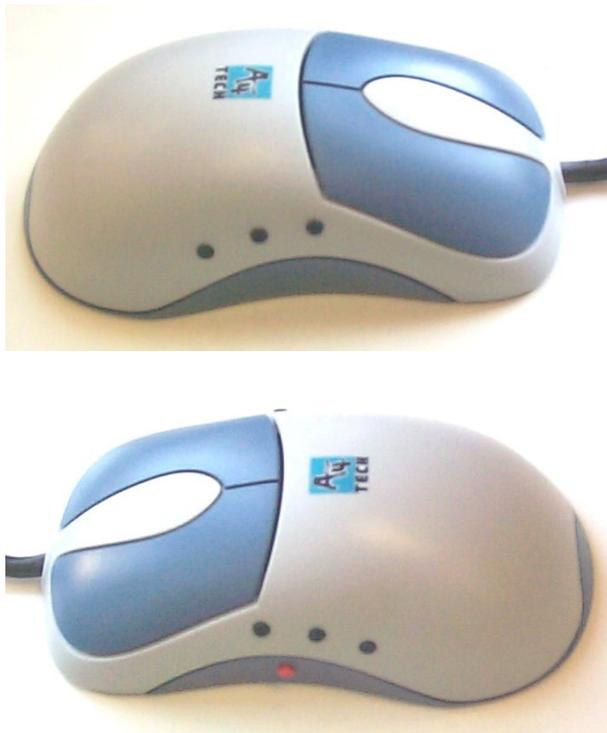
The optional mouse controller allows easy desktop access to the most commonly used front panel controls. These buttons are functionally equivalent to the corresponding front panel controls.
