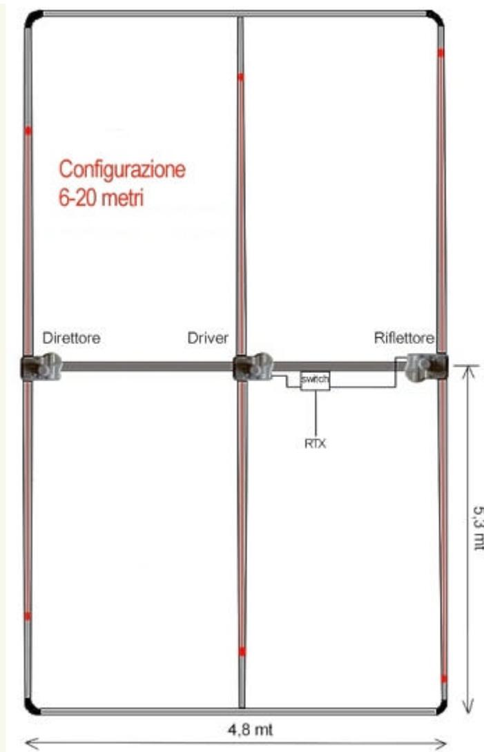
The UB-50 is a 3 element Yagi with two different radiating elements automatically switched by the Antenna Controller : a driven-element when used as a 3ele on 6-20mtr and a single radiator when operating on 30-40mtr. The same switching-system designed by UltraBeam and yet successfully used in our 6-40 mtr Yagis (3el and 4el models) was the most deciding factor of the ambitious UT-50 project.
