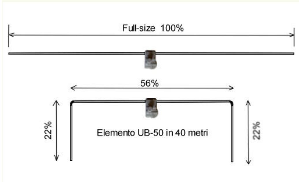
Our dynamic antenna system not only represents a multi-band antenna that has the ability to precisely adjust the length of each element (while in the air) to achieve the best performance in terms of gain and front to back ratio but, as you are probably aware, it also is the only system with the ability to better build different antenna-configurations and let them cohabit on the same boom and yet with utmost efficiencies.
