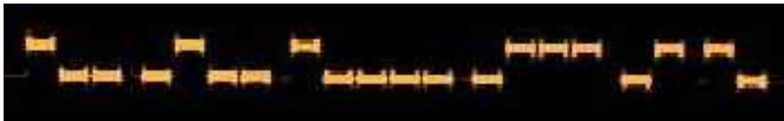
In DFCW mode all morse elements are of the **same length**. To distinguish DAHs from DITs, DAHs are shifted a few Hz upwards, i.e., DITs are assigned to the lower and DAHs to the higher frequency. Consecutive equal items are separated by small pauses of **1/4 dot length**. To produce this shift an external circuit is needed which is described later in this manual. The DFCW mode is switched on or off by the command **^D**, provided that a QRSS mode has been set before with **^S**.
