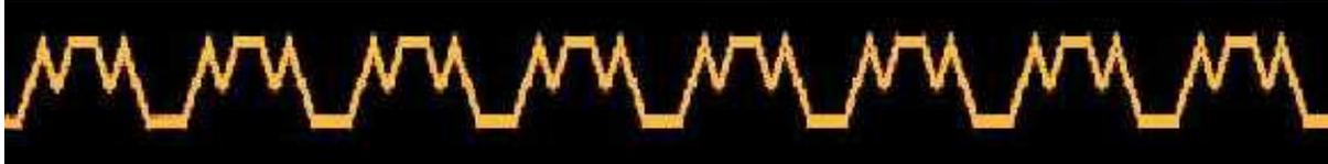
The commands **^F** and **^B** output falling and rising ramps whereas the **^J** command sets the binary counter which controls the D/A converter to a specified value. In combination with **^P** and **^T** arbitrary signal shapes can be generated.
