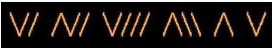
In SLANT mode CW elements are coded by slowly **rising (DITs) and falling (DAHs) ramps**.
