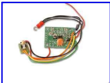
The [BHI NEDSP1061-KBD](http://www.bhinstrumentation.co.uk/html/nedsp1061-kbd.html) module (originally built for the YAESU FT-817 and the KENWOOD TS-50) can be used with the same great results on a YAESU FT-897D.
