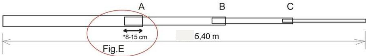
The glass fiber elements are formed by 4 telescopic sections. Its possible to extend every single conical junction to reach a total length of about 5.4m maximum extension. The length can change depending on the model.
