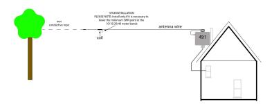
Please note: by varying the length of the wire located after the coil (short wire) you will influence the SWR of the 80 meters (3.6 MHz)
