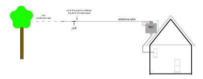
If you want to lower the operating frequency, install the supplied stub (see figure below) and adjust the length until you obtain the minimum SWR in the desired frequencies.
