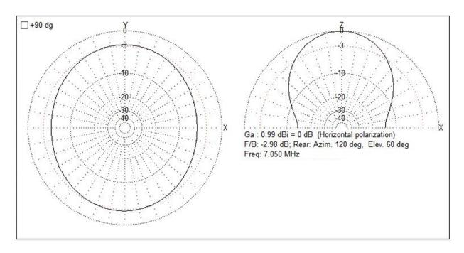
Figure 12. Horizontal NVIS Far Field Plot 7 MHz.
