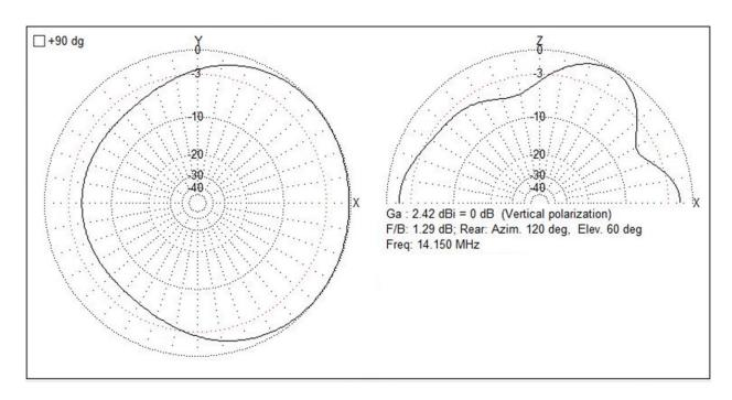
Figure 14. Inverted "L" Far Field Plot 14 MHz.
