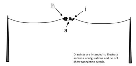
Figure (7). Horizontal Dipole.
