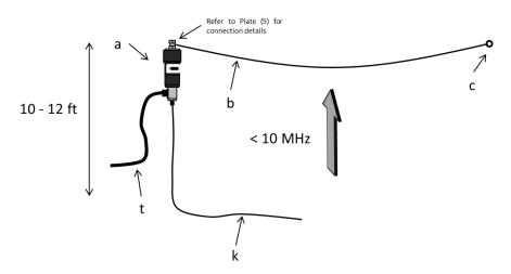
Figure 3. Horizontal NVIS Configuration.
