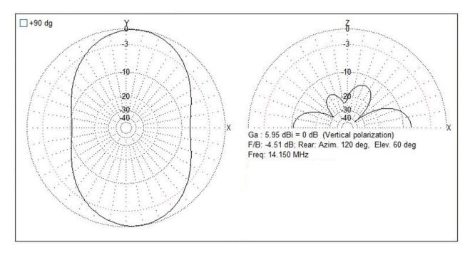
Figure 15. Inverted "V" Far Field Plot 14 MHz.
