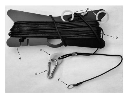
Plate 3. Antenna Wire Assembly.
