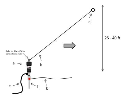
Figure 4. Sloping Wire Configuration.
