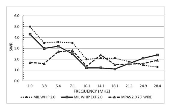
Figure 9. SWR by Frequency Graph.
