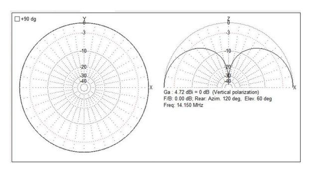
Figure 10. Manpack Vertical Far Field Plot 14 MHz.
