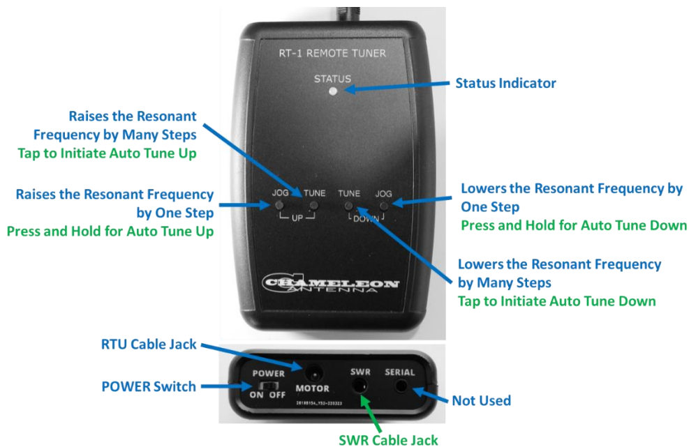
Plate 3. Remote Tuner Unit Controls and Connections Location.
