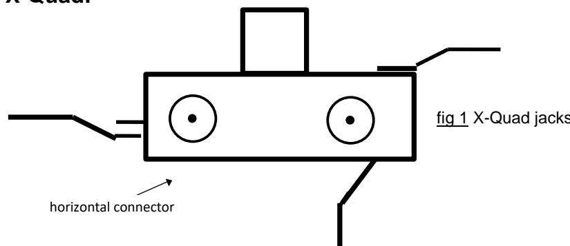
The antennas must be mounted with the N-jacks looking backward. The connector box must be horizontal. See figure 1.
