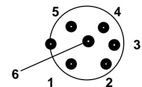
For switching apply 12V / 100mA to the correct pin. Without control voltage applied to any pin the antenna is switched to horizontal polarization.
