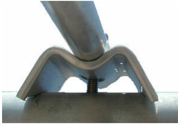
pic 5: don't tighten the elements screws more than shown!
