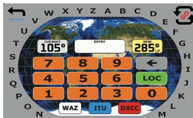
Figure 15 — The HEADING DIAL SCREEN allows you to enter the desired heading with the large on-screen keypad. It also allows you to set the heading for the QRA locator by specific DXCC country or prefix, or particular WAZ or ITU zone, to turn your antenna in the proper direction.
