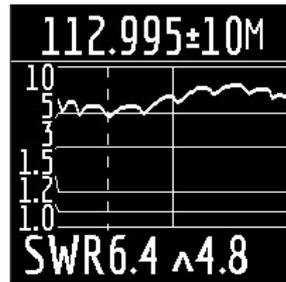
at the top of the screen: the value of the center frequency of the measurement and the width of the measurement band.
