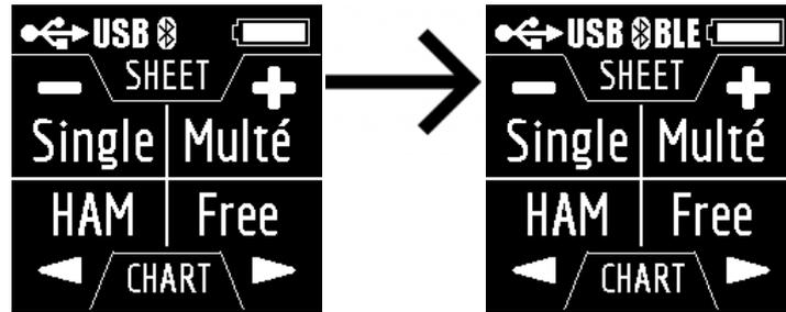
If the program could not detect the analyzer, check whether Bluetooth is enabled in the analyzer (1 mode in the Settings menu) and whether Bluetooth is enabled on your smartphone/tablet.
