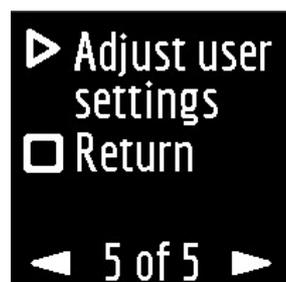
Pressing the key will take the analyzer to the **Settings menu**. Pressing the key will return the analyzer to the **Main menu**.
