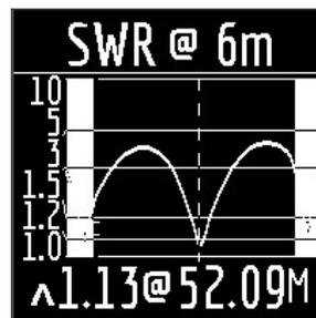
In **HAM mode**, the SWR icon and the range over which the measurement is carried out are displayed at the top of the screen.
