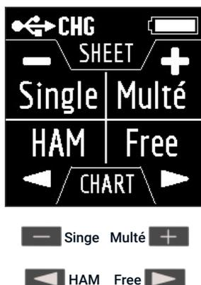
The **Single** and **Multé** functions display the measurement result as numbers, while the **HAM** and **Free** functions display the measurement results as numbers and charts.
