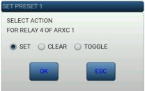
One of the options for Preset is the ARXC CONTROL window. In this window, **all** ARXC outputs can be observed and controlled from one place.
