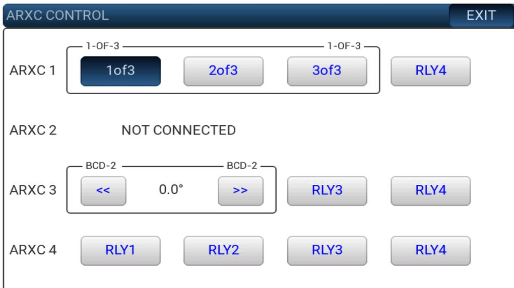
The indication and control is similar to that in Menu→System→ARXCx, except for the visual style (buttons instead of the "radiobuttons"), and the different handling of *BCD-N* groups. In ARXC CONTROL window they contain "forward/backward" buttons instead of individual relays control, and in between them, the current value, or, if azimuth control is enabled for given group, the current primary direction, is displayed.
