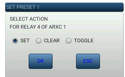
One of the options for Preset is the ARXC CONTROL window. In this window, **all** ARXC outputs can be observed and controlled from one place.
