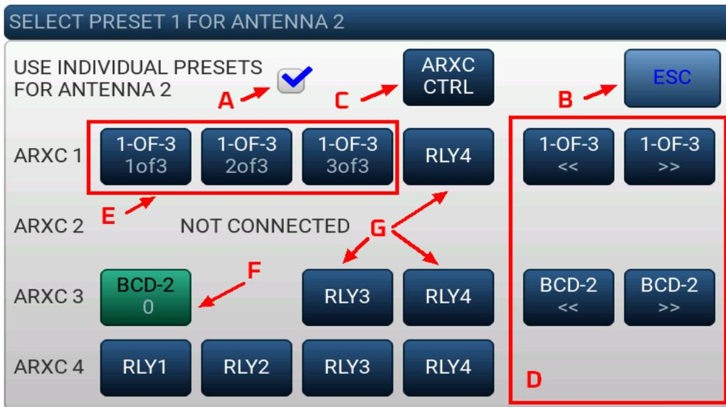
**A** - this tickbox determines, whether given Antenna has assigned an individual set of Presets, or, if unticked, uses the common set of Presets. Consequently, in this window, the individual or the common set of Presets is edited.
