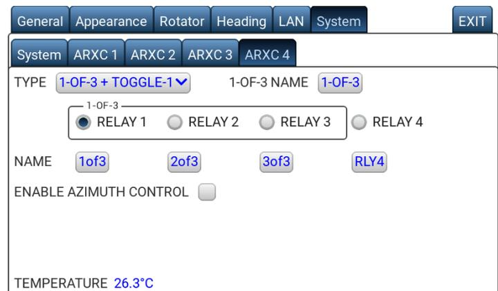
When azimuth control is enabled for 1-of-N by ticking the ENABLE AZIMUTH CONTROL tickbox, its menu slightly changes:
