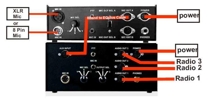
Connect the EQ-8 MIC OUT to the EQplus AUX INPUT using a 5-pin DIN to 5 - Pin DIN cable. (Power to both units should be OFF while connecting cabling.) Be sure to use the proper cable wiring. (Optional from W2IHY)
