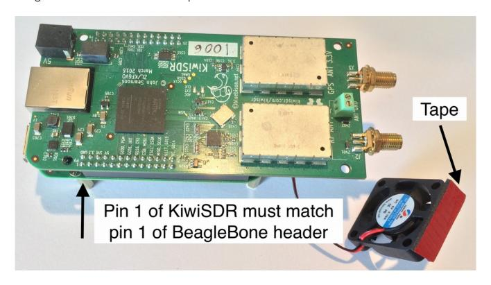
Flip Kiwi/Beagle over. Remove red protective paper from sticky tape. Stick fan to bottom of Kiwi board, offset as shown below, being careful to leave enough room for future insertion of an SD card (green arrow).
