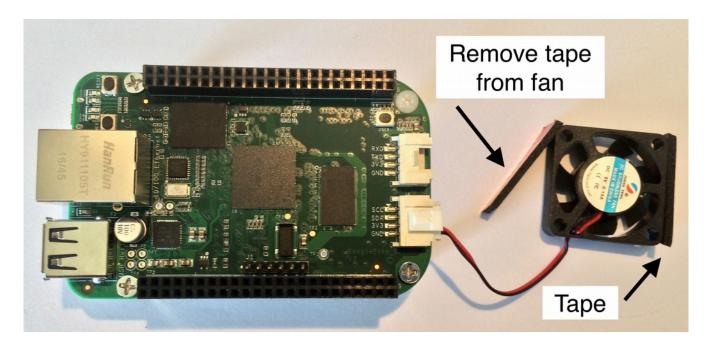
Plug KiwiSDR board into BeagleBone. **Be careful** to align the Kiwi board pins into the correct Beagle header sockets. The cutout in the Kiwi board should wrap around the Beagle Ethernet connector with equal clearance on all sides.
