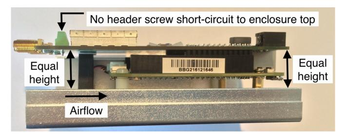
Place the top cover on the enclosure. Attach each end plate with four screws each. The antenna SMA connectors do not contact the enclosure because this was found to result in the lowest noise floor (i.e. grounding the SMAs would form a small ground loop with the Beagle-to-enclosure ground). Attach the four adhesive bumper feet to the bottom of the enclosure.
