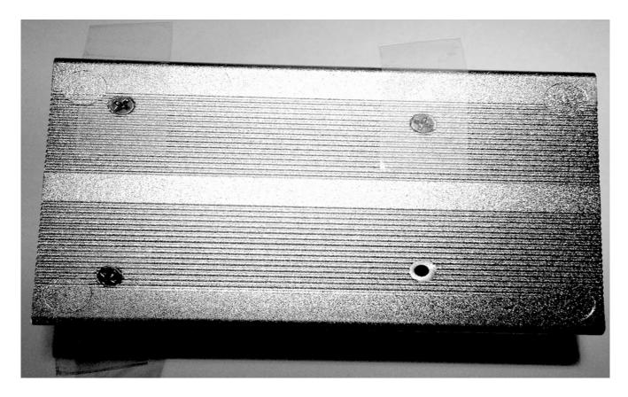
Invert the bottom enclosure piece and place one star washer on each screw thread.
