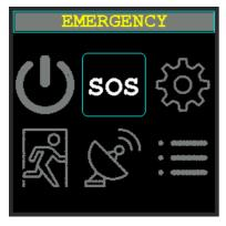
To send an "APRS EMERGENCY" (emergency) message, press and hold the center button for about 5 seconds.
