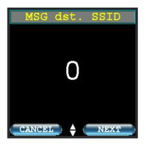
Use the up and down buttons to select an SSID between 0 and 15.
