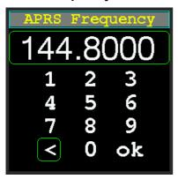
The frequency is preset to the usual US frequency of 144.3900 MHz and normally does not have to be changed.
