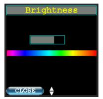
**Brightness** controls the display brightness. The gray bar shows the set brightness. Brightness is adjusted with the up and down buttons.
