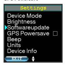
"GPS Powersave" defines whether the GPS receiver should be switched off automatically when GPS is not needed.
