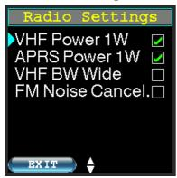
Here you can switch the **transmission power** in APRS or VHF operating mode between 0.5 or 1 watt. Green tick means 1 watt.
