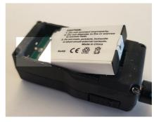
Insert in reverse order, please note the alignment of the battery contacts to the **contacts** in the PicoAPRS.
