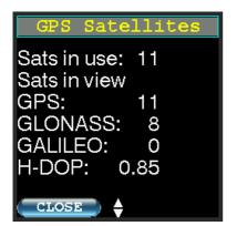
Sats in use shows the number of satellites actively used for position determination.
