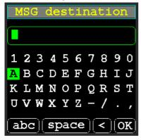
Enter the call sign and then the SSID of the recipient. To enter the SSID, you can confirm the selection "OK" (bottom right in the picture) or select the "hyphen" (-).
