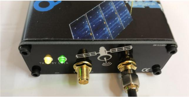
Fig 4 TX mode, TX/STBY led is Orange
