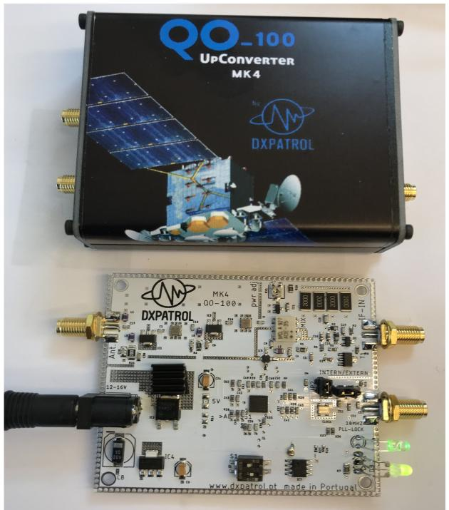
fig 1, Upconverter full assembled PCB
