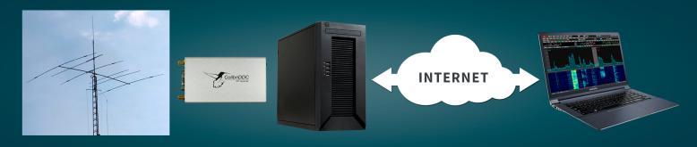
**Remote control system** - Expert Remote, utilizes a client-server connection. PC with the installed ExpertRemoteServer (**ExpertRS**) and connected to it ColibriDDC (one or several) used as a server. Server's PC connected to a router with an access to the Internet. PC with the installed ExpertRemoteClient (**ExpertRC**) used as a client.
