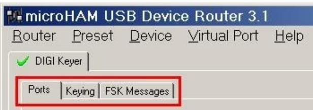
Router must be used to configure DIGI KEYER to function properly. The device configuration tab (in the red rectangle) is used to setup each part of the DIGI KEYER – virtual ports for communicating with the application (Ports), audio levels, PTT and keyboard FSK (keying), and stored FSK messages (FSK Messages).
