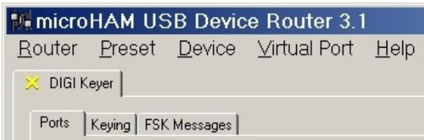
When Router shows a **YELLOW** "X" insted of a green ✓, it means the USB driver is correctly installed but DIGI KEYER is not receiving power from the radio or external supply.
