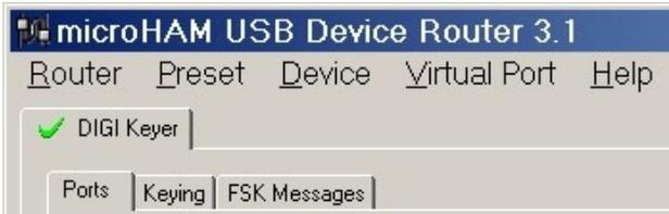
When the USB driver is installed correctly and DIGI KEYER is powered from a radio or external 12V DC supply Router will show a device tab with a **GREEN** check beside the device name (DIGI KEYER).
