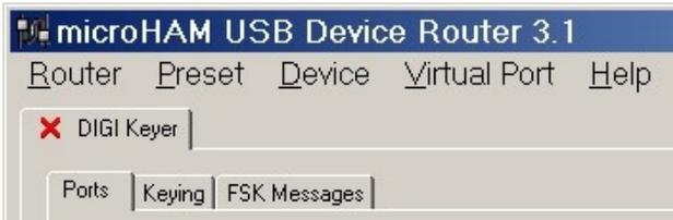
When Router shows a **RED** "X" insted of a green ✓, it means the device is disconnected and Router does not see the USB part of DIGI KEYER.
