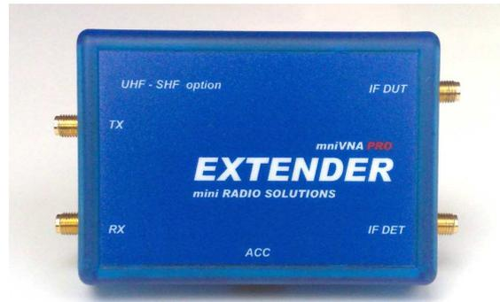
The **EXTENDER** is designed to be connected to the **miniVNA PRO** using the two SMA connectors marked **IF**. The unit is powered from the **miniVNA PRO** via the accessory port by a common CAT5 cable (supplied).
