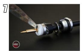
Insert one of the two teflon discs and subsequently the central pin. Solder the pin to the inner conductor, inserting tin in the provided hole. Avoid heating the pin for a too long time in order not to damage with excessive heat the cable dielectric (which is not made in teflon!)
