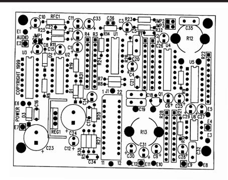
C1,C3, C4,C6,C14, C25-C28, C33 4.7 uF radial electrolytic R1, R2, R22 - 10K ohm 5 Resistor 10 pin SIP C7\*, C13\*, C16, C17, C32 .1 uF ceramic monolithic
