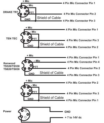
DIN connectors shown on the side to be soldered DO NOT SOLDER TO SHIELD OF DIN
